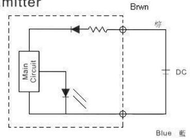
DC 3 Wires through beam type PNP NO\NC
